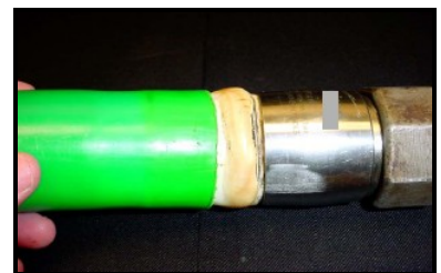
Flexible piping is bulging
